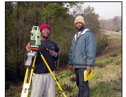
An important early step in any PD&E study is to obtain an accurate survey of existing boundaries in the study area. Lucious Andrews, III (left, with survey instrument) and Shantell Ingram, of Diversified Design & Drafting Services, Inc., are pictured during their survey work for the Capital Circle NW/SW Study. This work included the boundaries of the road's right-of-way line, as well as property lines and the exact location of other important features in the landscape, such as wetland edges and railroad boundaries.
